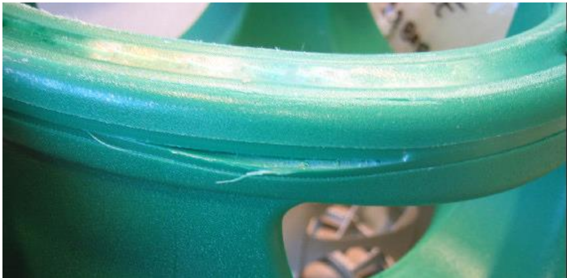
Figures 2 and 3: Unacceptable outer casing damage
